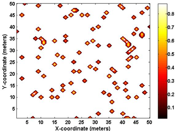
Fig. 5. Residual energy distribution in the sensor network, using the normalized CHEF protocol, with modulation diversity. The proposed scheme presents an energy-balanced performance along the network.
