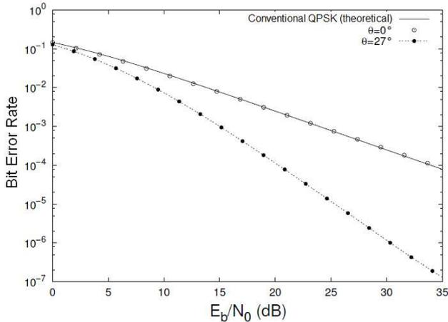
Fig. 1. Bit error rate for the modulation diversity scheme.
