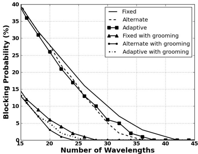
Fig. 5. Blocking probability versus number of wavelengths for the NSF network.
