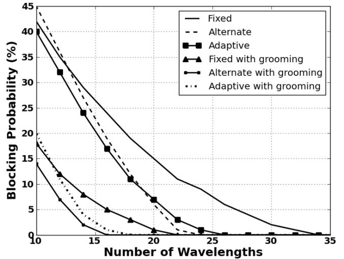
Fig. 4. Blocking probability versus number of wavelengths for the mesh-torus network.
