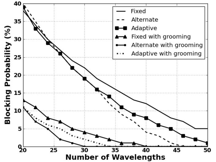
Fig. 3. Blocking probability versus number of wavelengths for the simple mesh network with five nodes.
