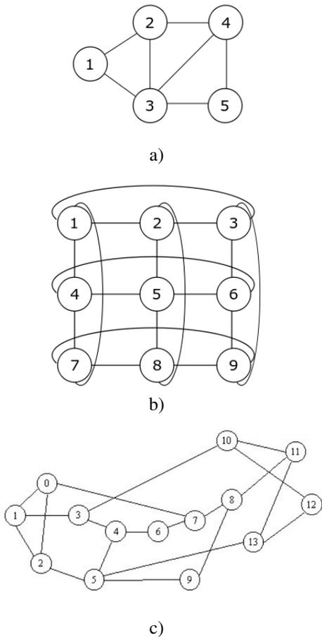
Fig. 2. Topologies used in the simulation: a) simple mesh network with five nodes, b) mesh-torus network and c) NSFNet.
