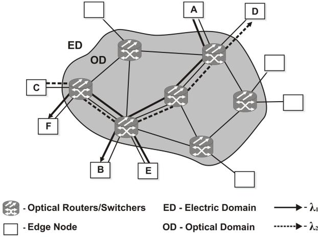
Fig. 1. Representation of an optical network.
